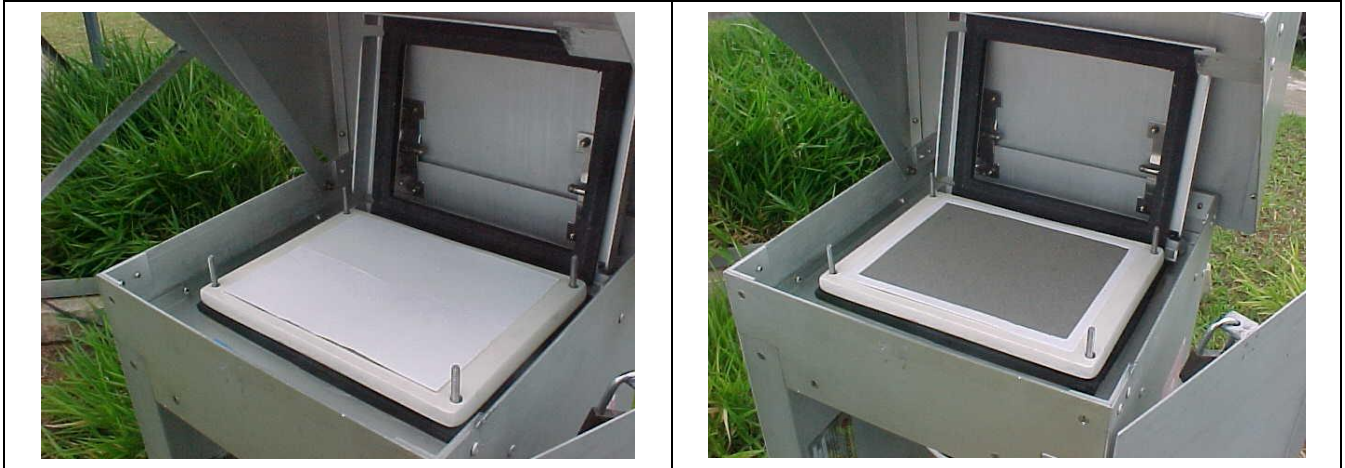
Figure 5 – Typical filter, before and after the collection.
