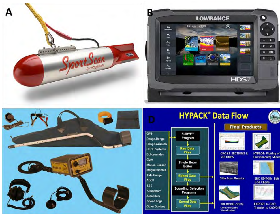
Photograph No. 2.11 Remote sensing equipment to be used in the marine archaeological survey. A. Side Scan Sonar Imagenex, SportScan model (imagenex) B. Echo sounder with side scan image, Lowrance model HDS 7 Gen 3 Structure Scan (Lowrance) C. Manual metal detector, model JW Fishers, Pulse 8x (JW Fishers ), D. Navigation software Hypack survey (Hypack)
