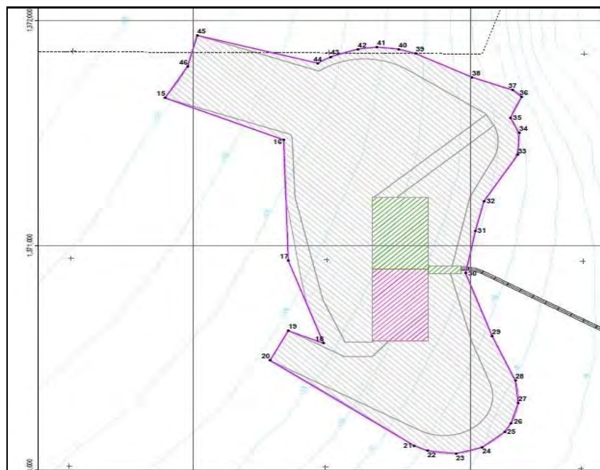
Figure No. 5.38 Polygon of dredging area and installation of the dock. Source: Prepared by Aqua & Terra Consultores Asociados S.A.S
