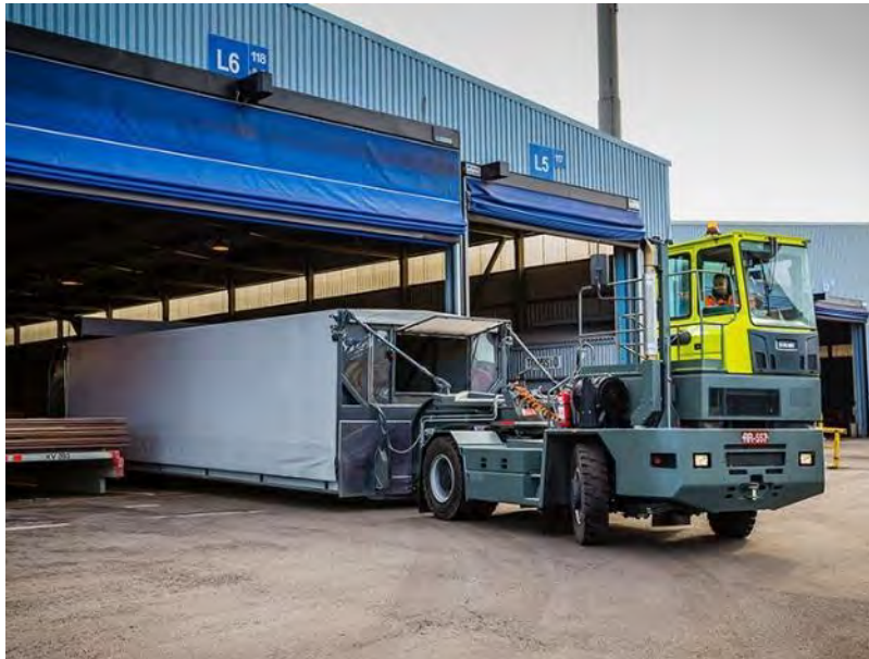
Figure No. 5.244 Kalmar equipment TR626i / TR632i Transport vehicle that will transit the viaduct.
