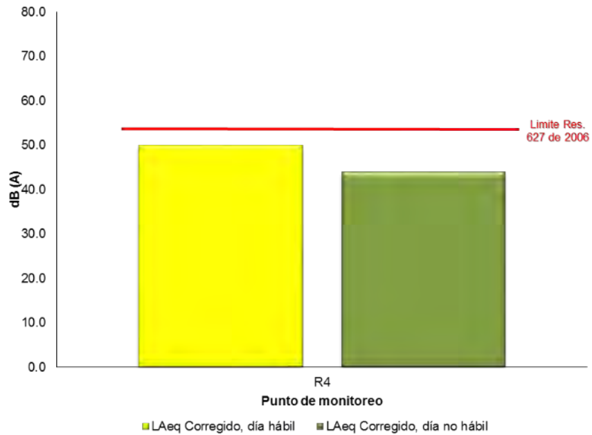
Monitoring Points----Corrected LAeq(working day)-- Corrected LAeq(non-working day) Figure No. 5.242 Environmental noise at night time, monitoring point R4 Source: SGS COLOMBIA S.A.S., July 2015
