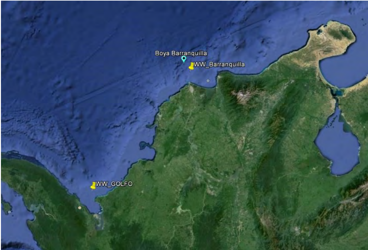
Figure No. 5.264 Sites with information related to waves from the WaveWatchIII™ project. The point WW_Barranquilla correspond to the series of WaveWatchIII™ that was used to calibrate the data of the model with the data of the Barranquilla buoy and the point WW_GOLFO is the series used to obtain the average regime in indefinite depths.
