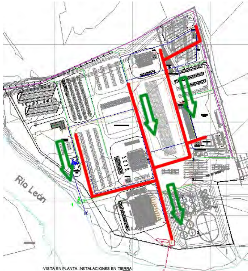
Figure No. 7.7 Behavior of domestic wastewater networks projected on land, with green arrows for the direction of flow
