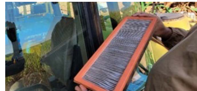
Activated carbon filter responsible for the air quality in the cab of the self-propelled sprayer.
