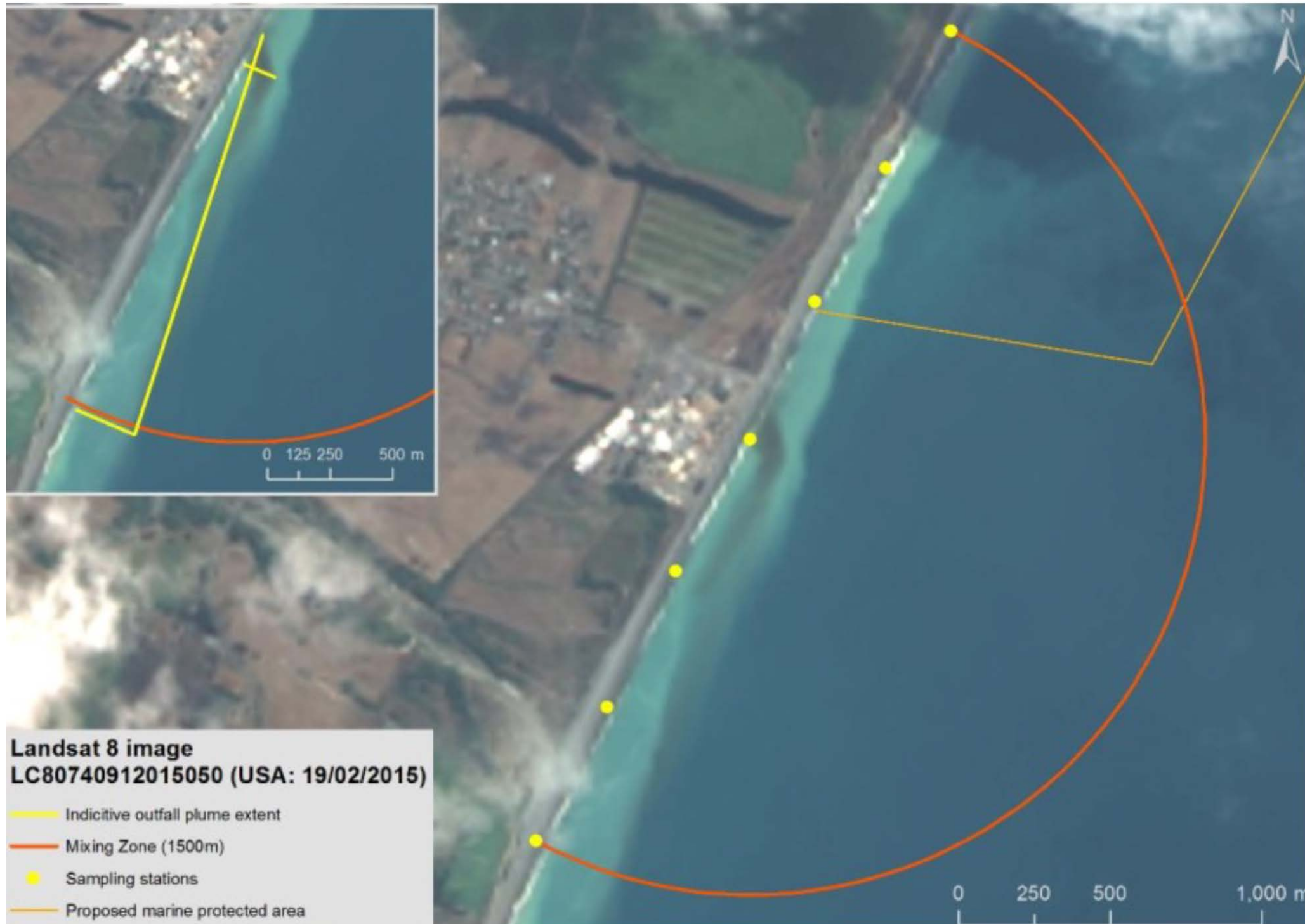
FIGURE A-4.2 Landsat 8 satellite image (captured USA time: 19 February 2015) shows a diffuse plume extending to the south, slightly beyond the mixing zone boundary.
