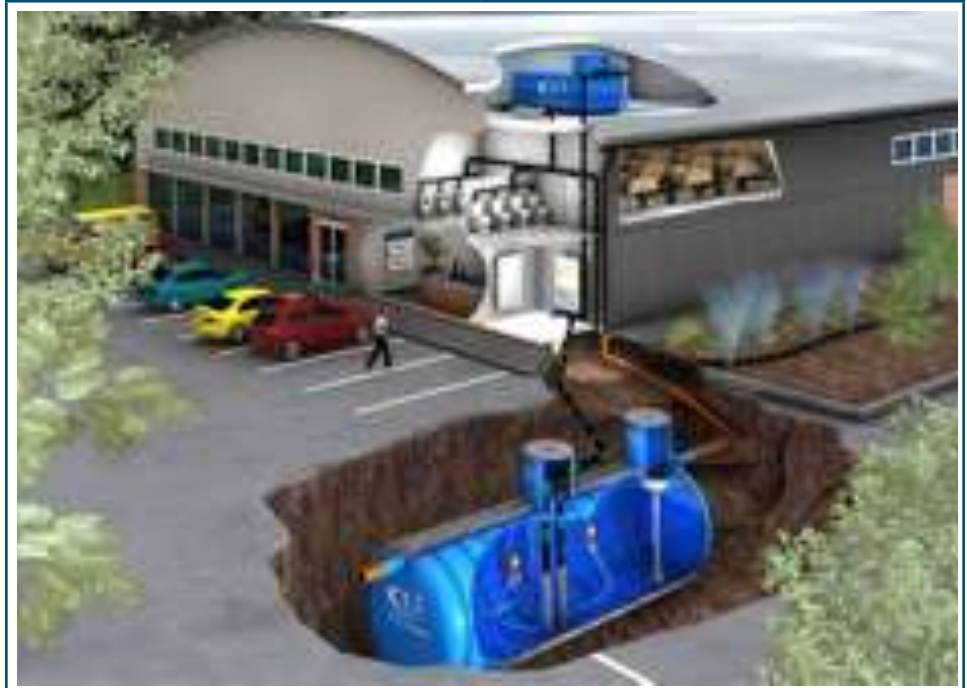
Figure AA: Collection of water into water storage tanks.
