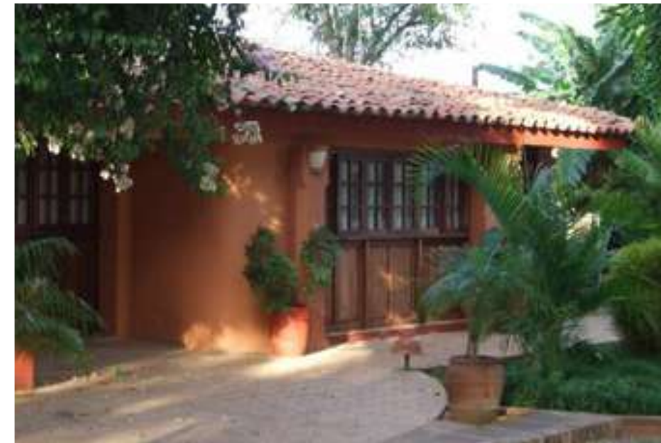
Reducing sunlight exposure to walls using natural shading such as plants or a high fence
