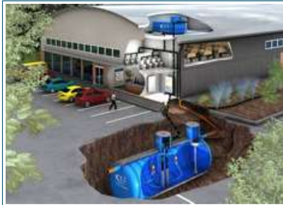
Figure AA: Collection of water into water storage tanks.
